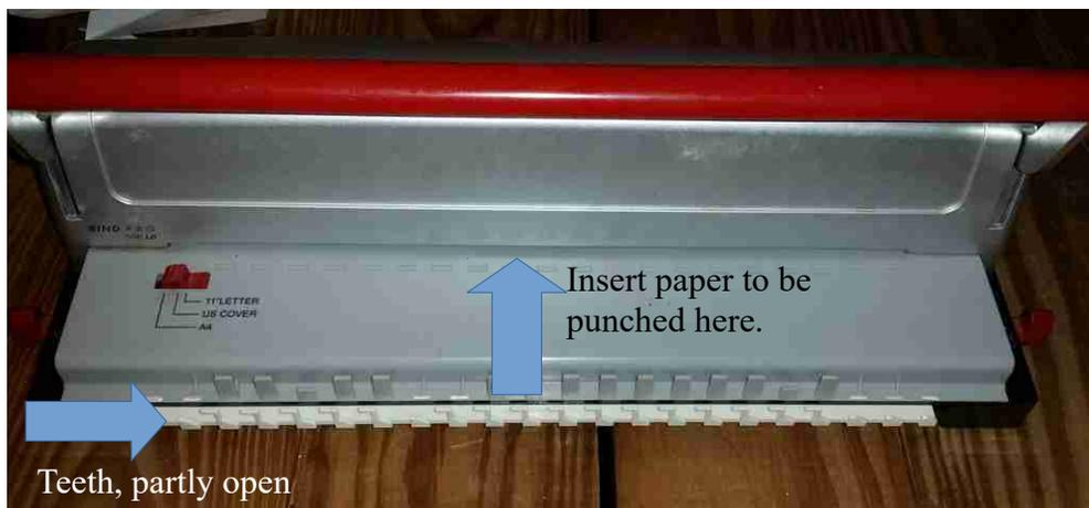
Black plastic spine inserted, and teeth holding spine ribs open. Insert punched edges of paper from above, so pointed ribs of spine line up with holes. Slowly close teeth using red knobs, so spine points move through holes in paper.
