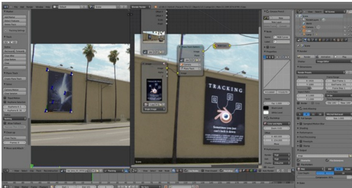
Above: Motion Tracker feature in Blender v2.69 can replace billboards in video footage.
